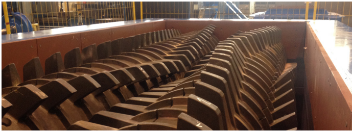
Sizer SWB0740, rotor diameter 700 mm, rotor width 4000 mm, coal 2500 t/h
